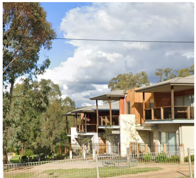
Dwellings designed with habitable rooms and windows overlooking adjacent public open space providing passive surveillance opportunities.
