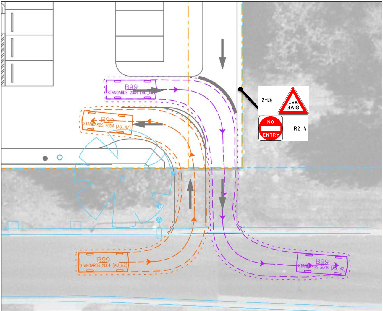
Figure 11 Proposed Car Park/Roadway Interface Signage and Linemarking
