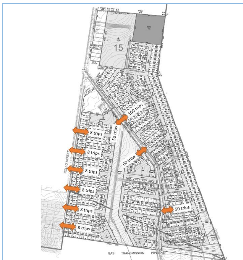
FIGURE 11: TRAFFIC GENERATION TO EXTERNAL ROAD NETWORK
