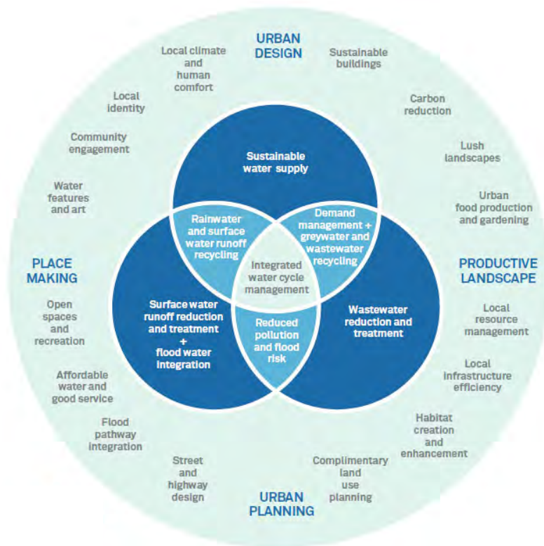
Figure 2 Integrated water management diagram showing the interaction of the three 'areas' of water management within a context of urban form and landscapes.
