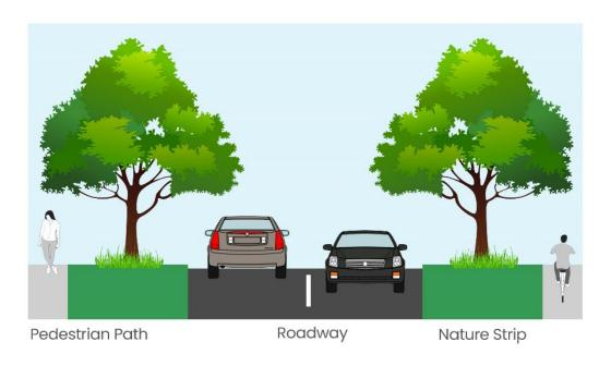
Figure 1: Typical Cross Section of Nature Strips
