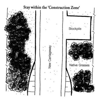
Figure 8. Clearly identify area of disturbance or machinery access or 'Construction Zone'.
