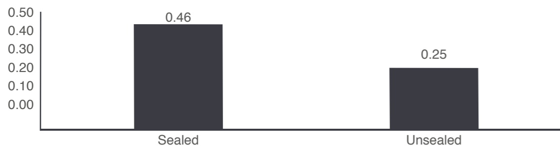
Figure 30: FSI Crashes per Kilometre of Sealed and Unsealed Road
